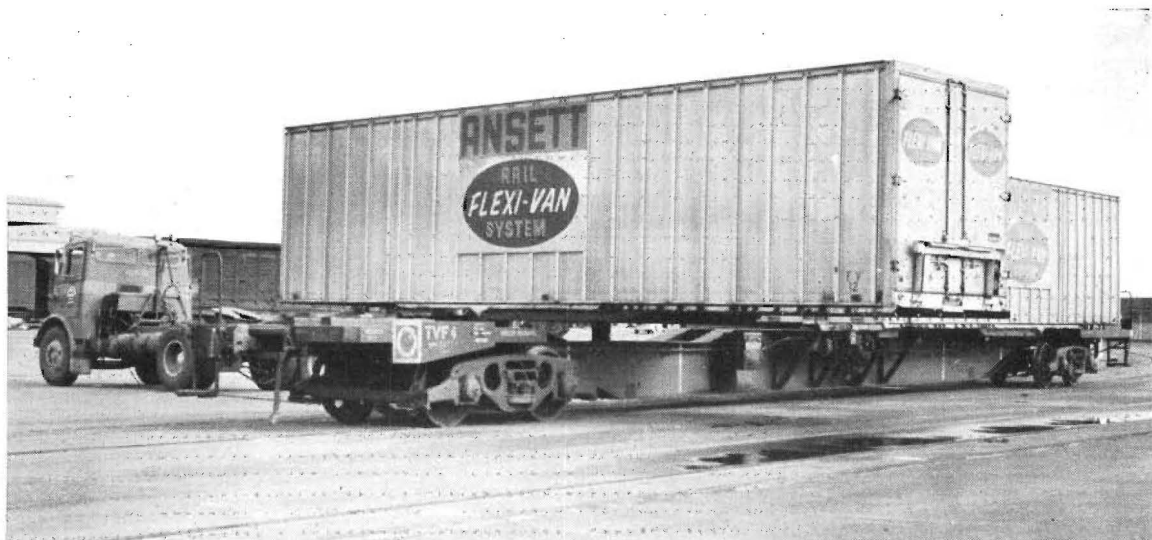
Loading a " Flexi-van " unit on one of the wagons specially constructed for this type of traffic between Melbourne and Sydney.
