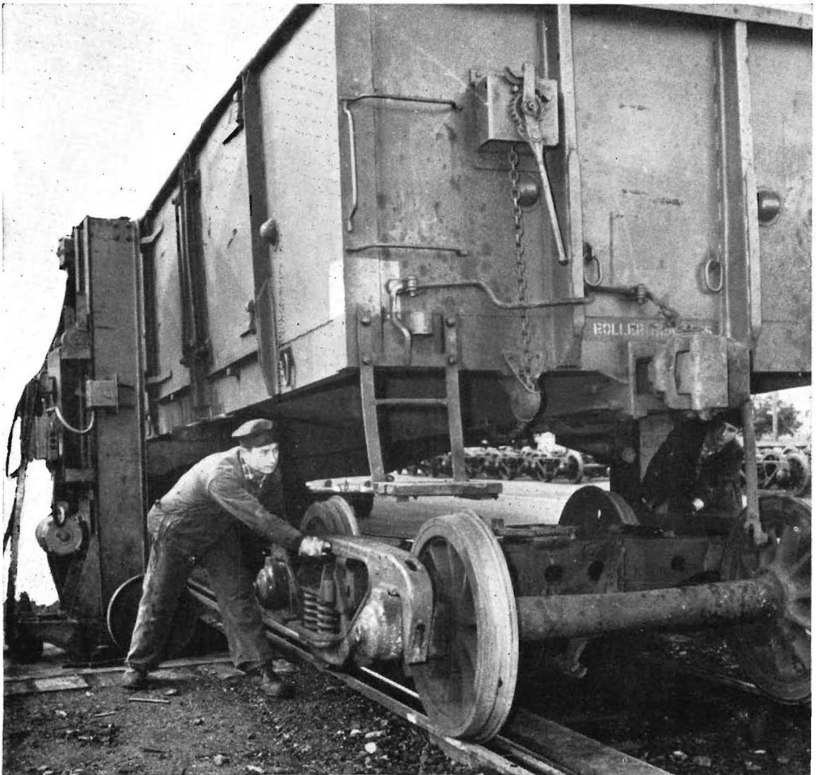
Bogie exchange procedure in operation at Dynon.
